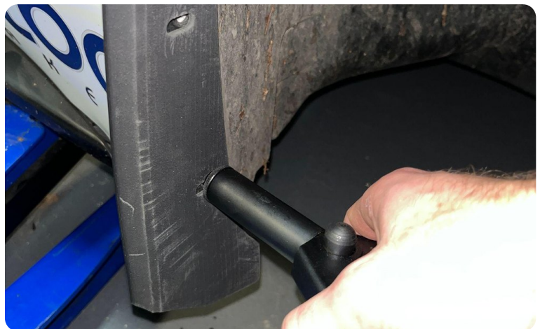
SET EACH REPLACEMENT RIVET WITH THE INSTALLATION TOOL
