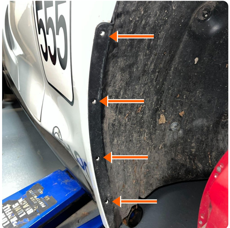
REMOVE THE FOUR FACTORY RIVETS
